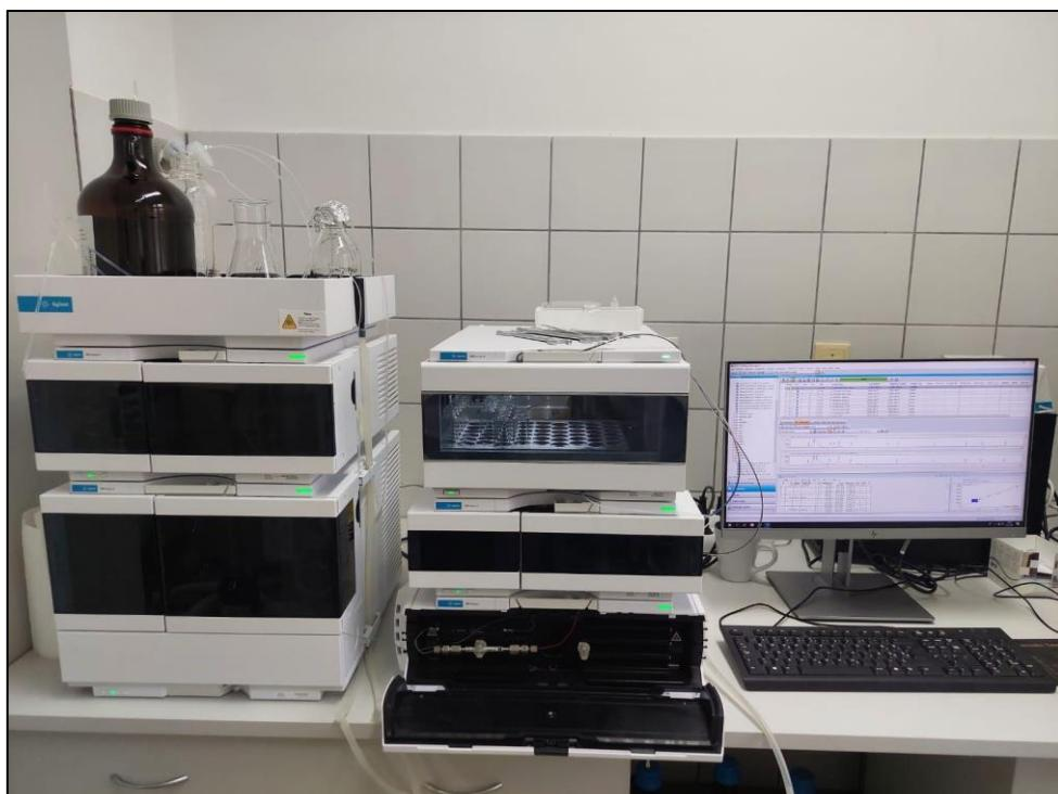
Slika 2. HPLC uređaj; Agilent technology 1260 Infinity II
