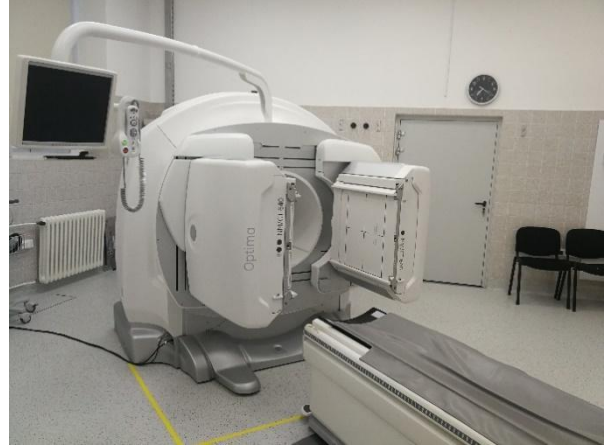
Slika 2. GE Healthcare Optima NM/CT 640 SPECT/CT (izradila autorica)
