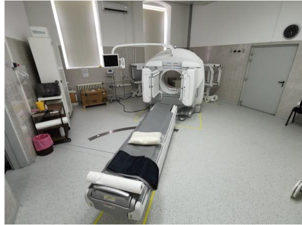
Slika 3. GE Healthcare Optima NM/CT 640 SPECT/CT (izradila autorica)
